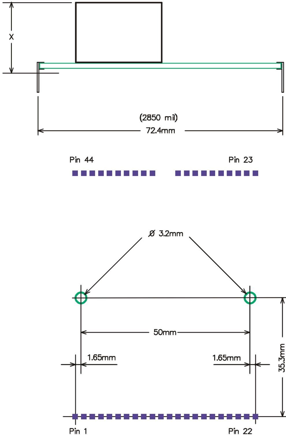
Fig. 3 Side view (top) / Mechanical fixing (bottom) 2SD315A
