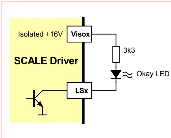
Fig. 6 Status display with LED at pin LSx
