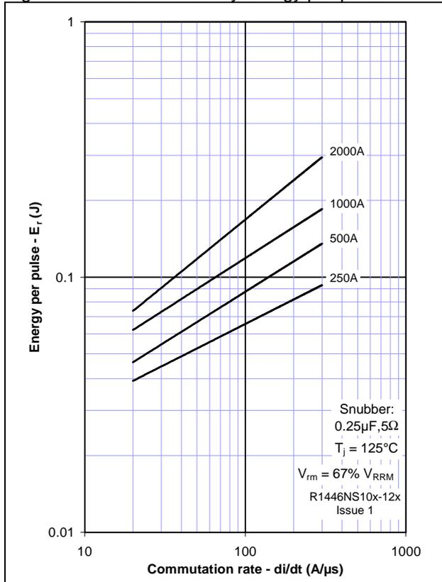
Figure 10 - Sine wave energy per pulse
